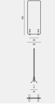
AK 3 is a functional room divider for commercial interiors. The divider creates movable walls, bringing structure to open spaces. Made from PET Felt and honeycomb paper core, AK 3 has acoustic properties and is an effective solution for dampening the noises. The divider offers a wide range of applications in open-plan offices, restaurants and other public places.
