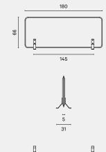
AK 4 is a functional workplace divider for commercial interiors. The divider creates partitioning at shared desks, allowing people to work in a concentrated manner. Made from PET Felt and honeycomb paper core, AK 4 has acoustic properties and is an effective solution for dampening the noises. Suitable for open-plan offices, co-working spaces and other public interiors.
