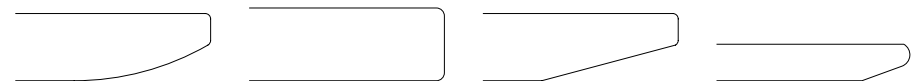
Solid wood edge, rounded on the bottom, plastic liping straight, chamfered wood edge or HPL solid core, chamfered edge
